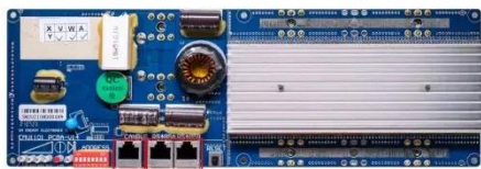
RS485 Communication between one battery and inverters Band rate: 9600bps RS485 Interface Communication between parallel packs of BMS and PC Band rate: 9600bps
