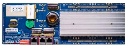
RS485 Communication between battery and inverter Baud rate: 9600bps RS485 Interface Communication between parallel packs of BMS and PC Baud rate: 9600bps
